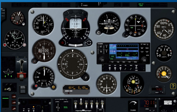
Pilot's control panel L-39
