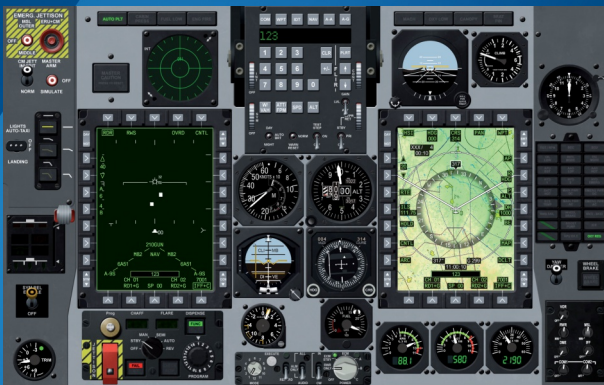
Pilot's control panel L-159
